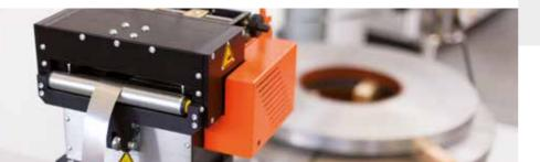
BRUDERER automatic stamping machine with draw-in feed for the manufacture of highprecision mass parts
